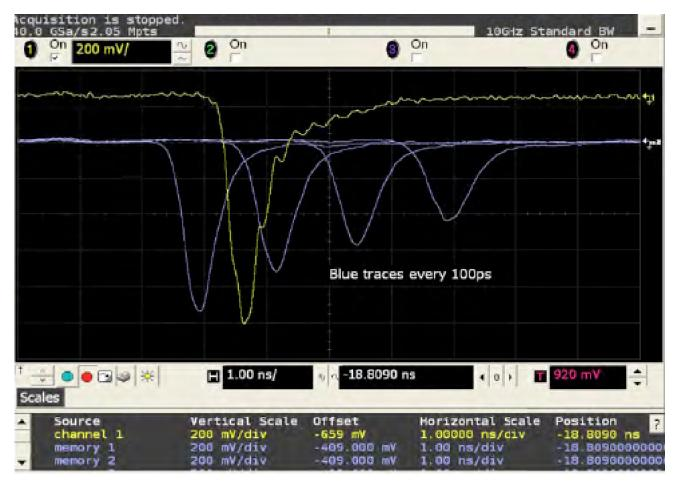
This figure shows the record of the output from a 40ps laser diode pulse, with resolved structure down to ~20ps. The four blue traces are used to calibrate the time base in dilated space. They represent 100ps intervals between them although their separation is shown here at 1200ps giving a diation factor of ~ x12.
