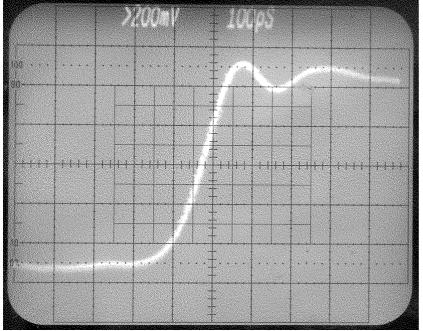
Showing risetime and jitter T rise ~130psecs Jitter <10ps rms
