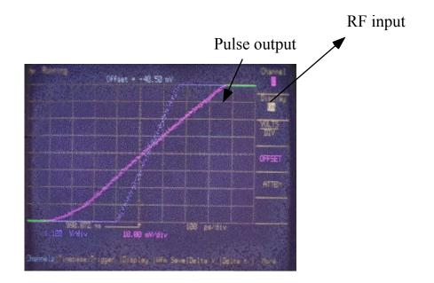
Showing the jitter with respect to 500MHz input (approx 10ps RMS)
