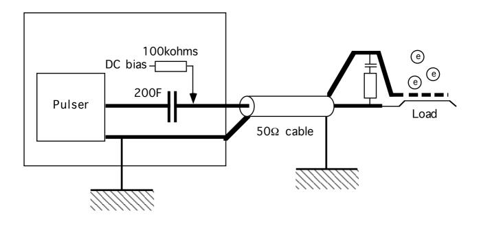
There is a resistor in series with a capacitor shown at the electron gun to make the load close to  $50\Omega$ . This must be chosen to minimise reflections up and down the connecting cable. (A typical value is  $100\Omega$ ).
