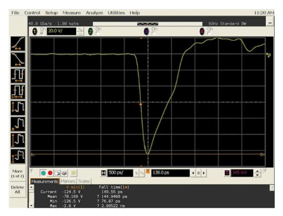
Max amplitude, 10MHz internal trigger, Barth 142
