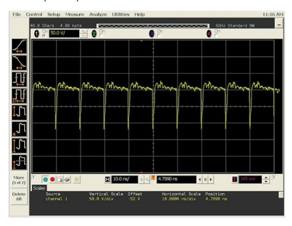
Max amplitude, 100MHz internal trigger, Tenuline 8340-200
