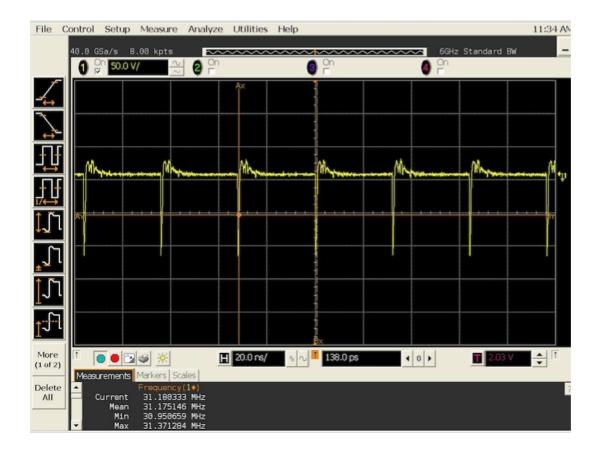
Internal /1 mode, minimum fine rate (~31MHz)
