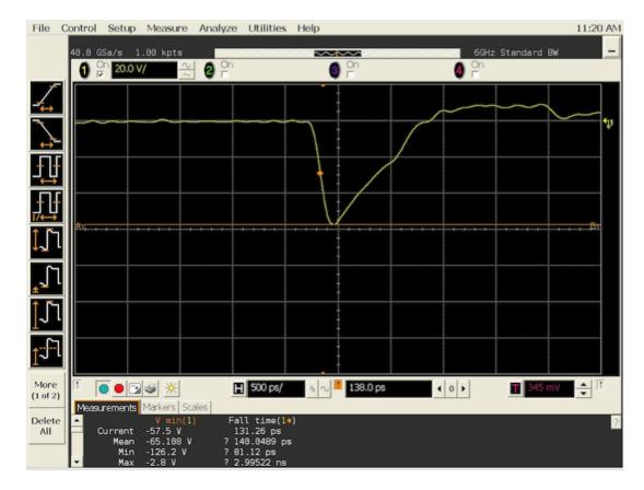
Min amplitude, 10MHz internal trigger, Barth 142
