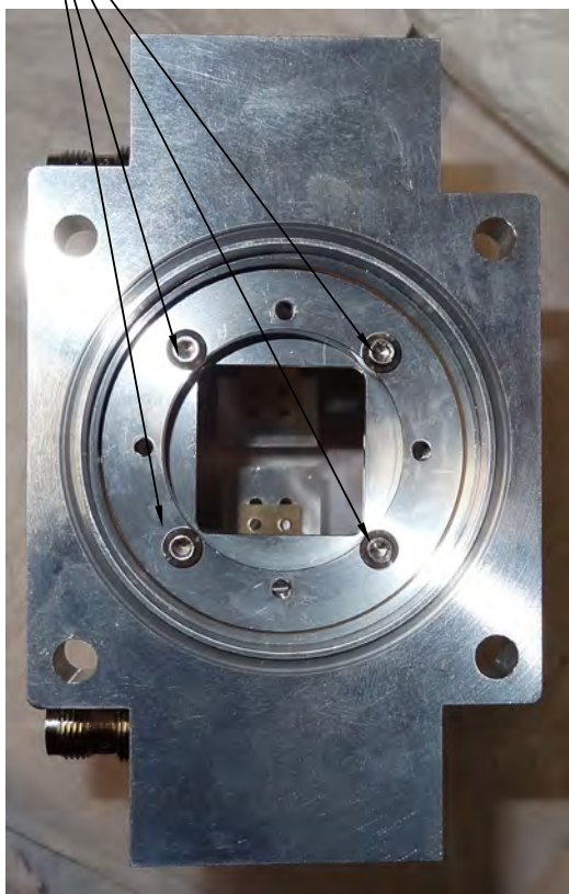
Figure 6 The scrapper ring can be loosened and moved. If necessary it can be mounted in the reverse direction using the second set of threaded holes.
