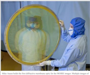
Mike Aasen holds the first diffractive membrane optic for the MOIRE imager. Multiple images of Tom Carlson appear behind the optic, which was designed and verified to achieve greater than 30 percent efficiency for the image used by the telescope.
