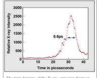
The time history of the X-ray emission from an experiment demonstrating sub-picosecond X-ray gating measured by the Dilation X-ray Imager.
