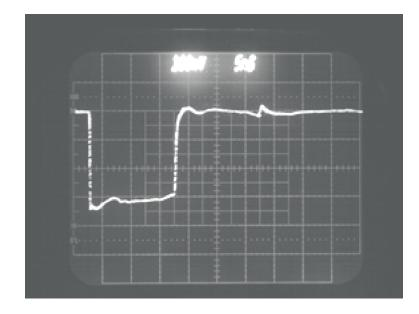
Vertical: 1kV / div. Horizontal: 5ns / div. Rep. rate: 10Hz
