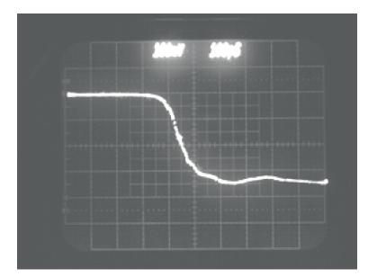
Vertical: 1kV / div. Horizontal: 100ps / div. Rep. rate: 10Hz
