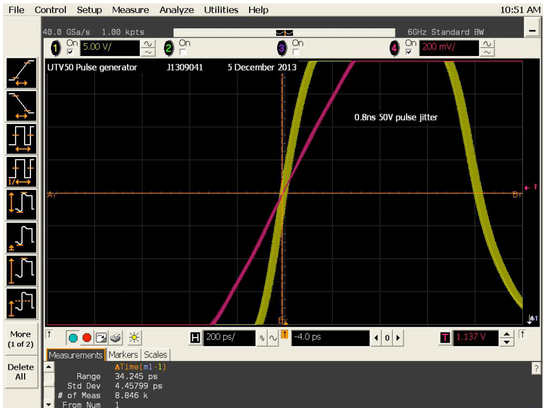
Figure 7 Pulse jitter with minimum pulse width
