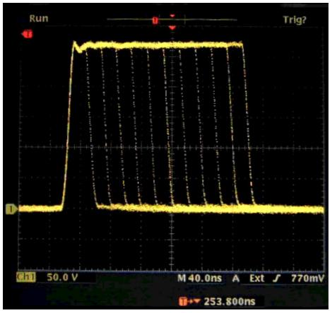
Pulse widths between 30ns and 200ns
