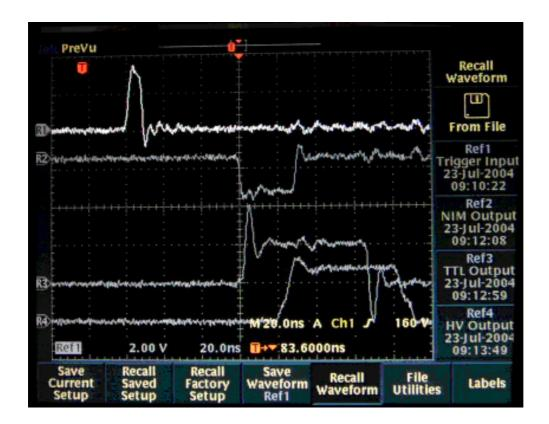
Showing the relative timing of the trigger, monitor and HV output signals at the front panel.
