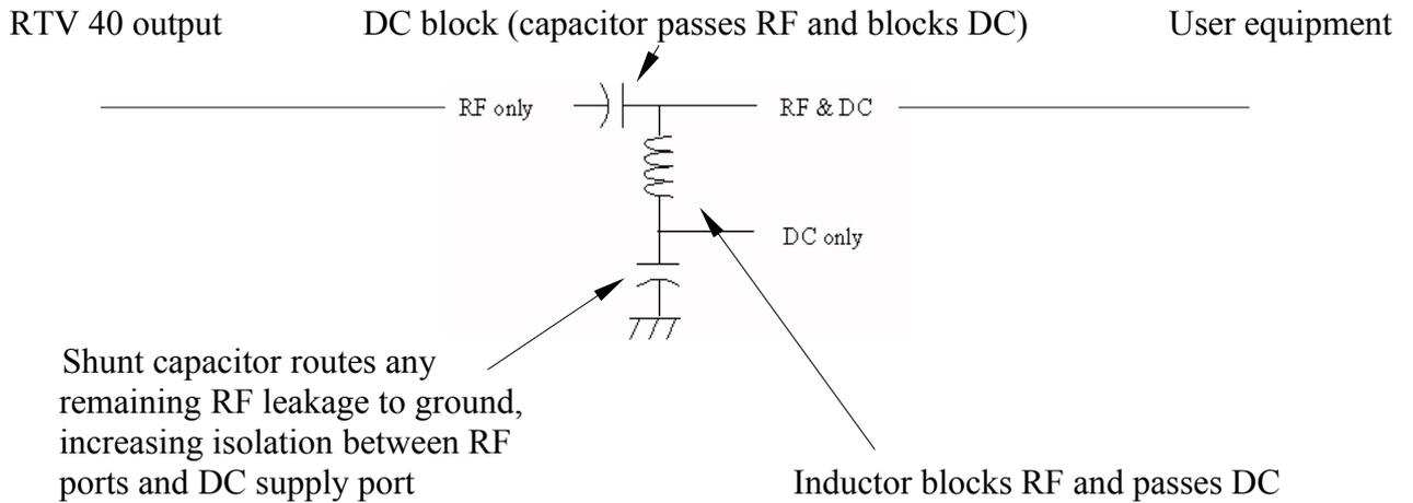
Alternatively, a Bias Tee can be used. This is a fully connectorised unit with the dc injection port built in.
