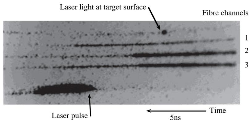
Figure 1. Typical Streak data showing three fibre channels extinguishing plus two fiducials of the incident laser pulse.
