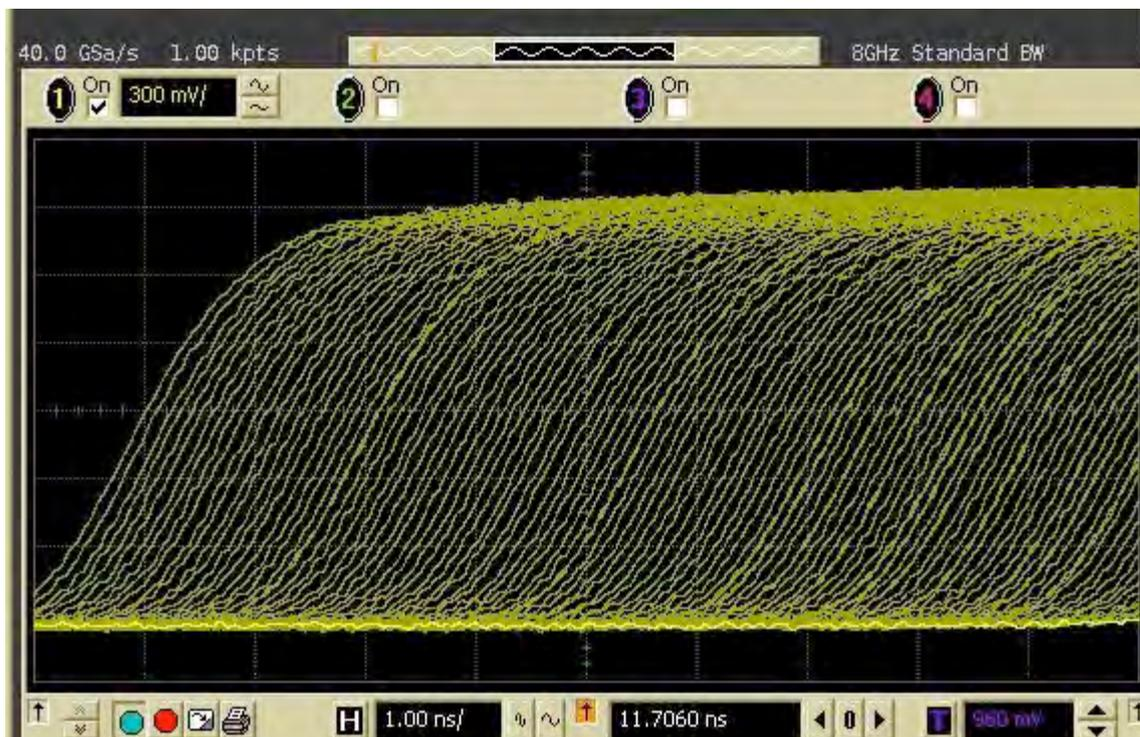
Figure 4 100ps delay increments from zero.
