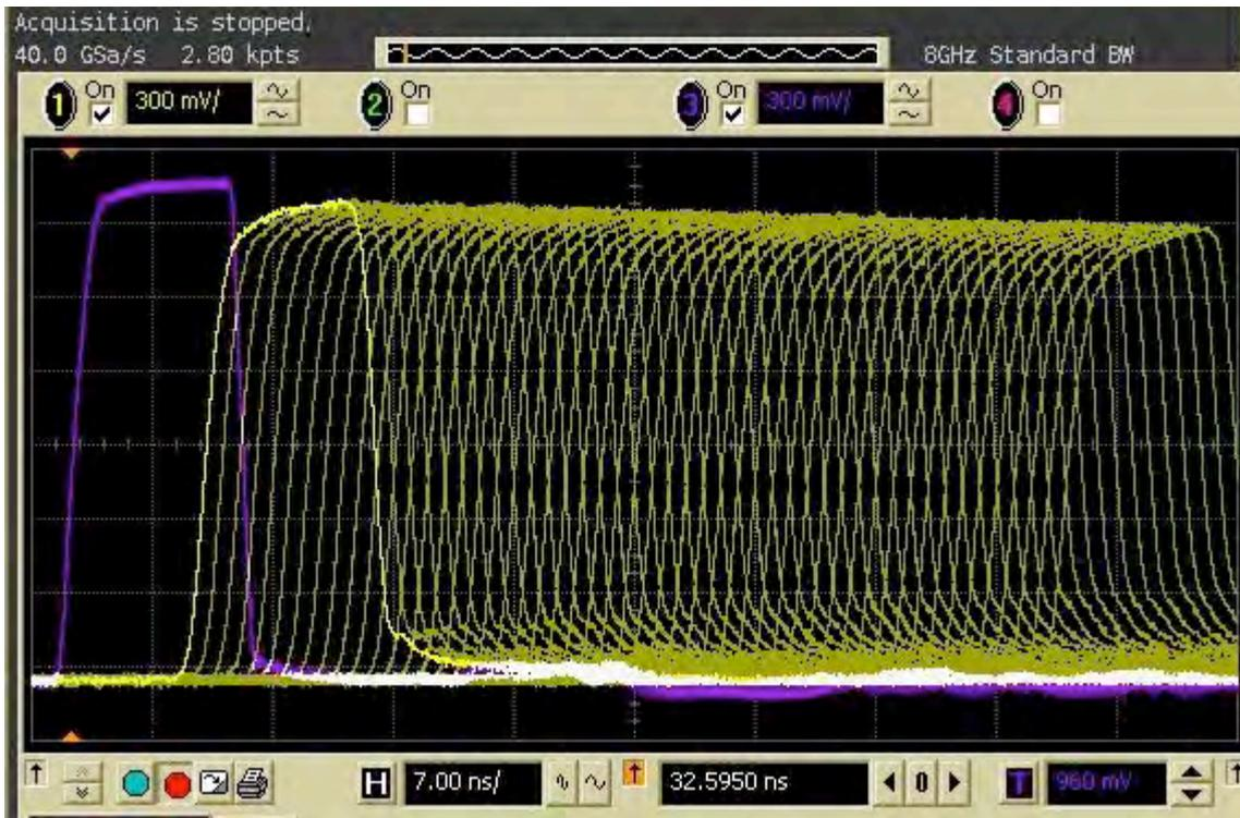
Figure 3 Delay with 1ns increments.
