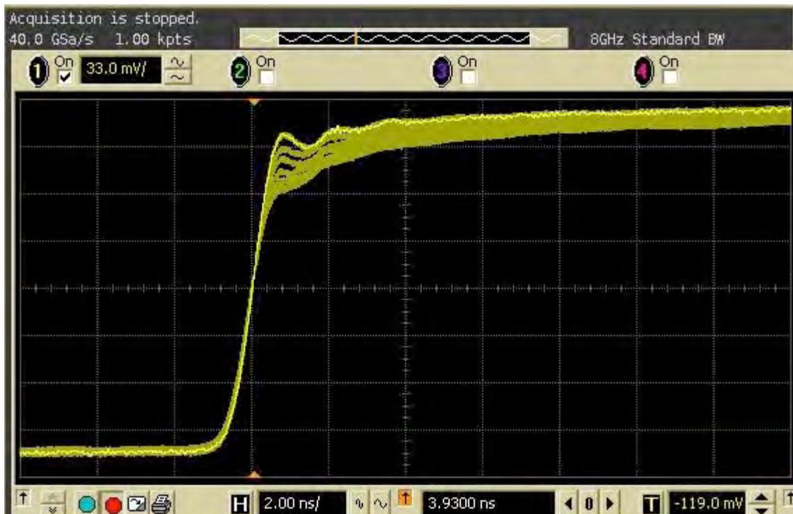
Figure 6 Degredation of rise tim eof a pulse as the delay is increased.
