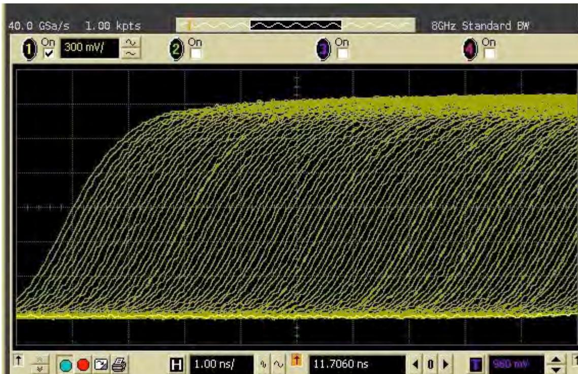
Figure 4 100ps delay increments from zero.
