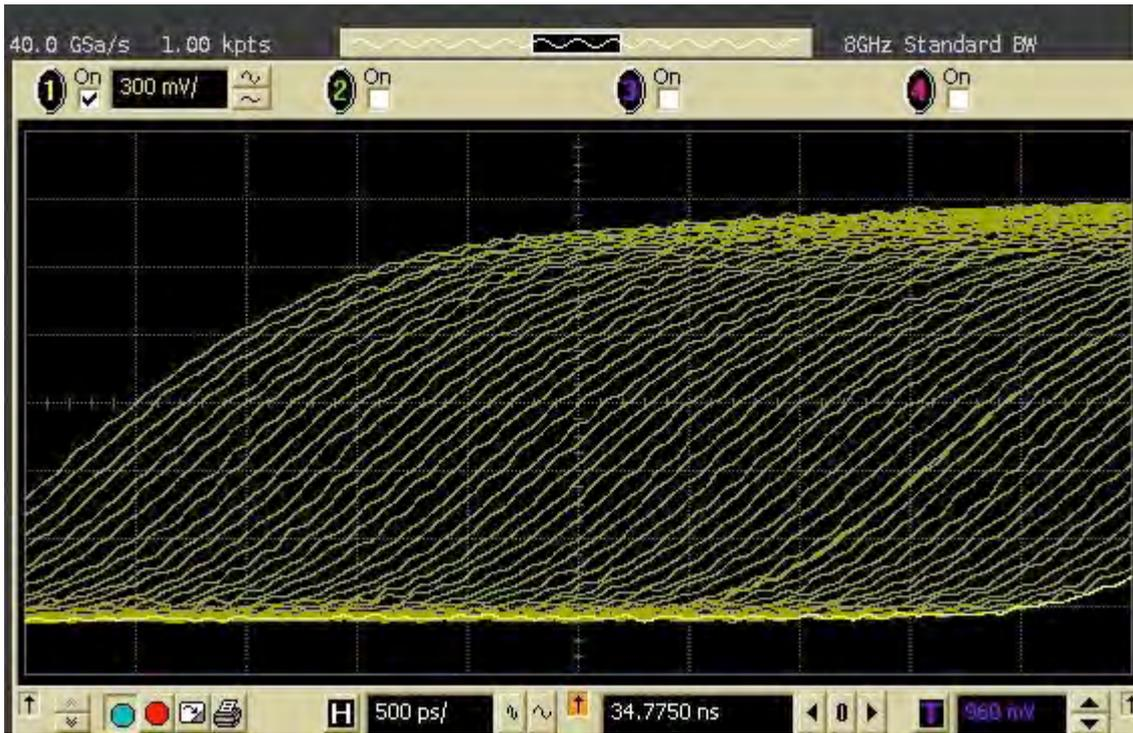
Figure 5 100ps delay increments from 25ns.
