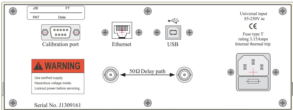
Figure 1 The rear panel showing the input and delayed output.
