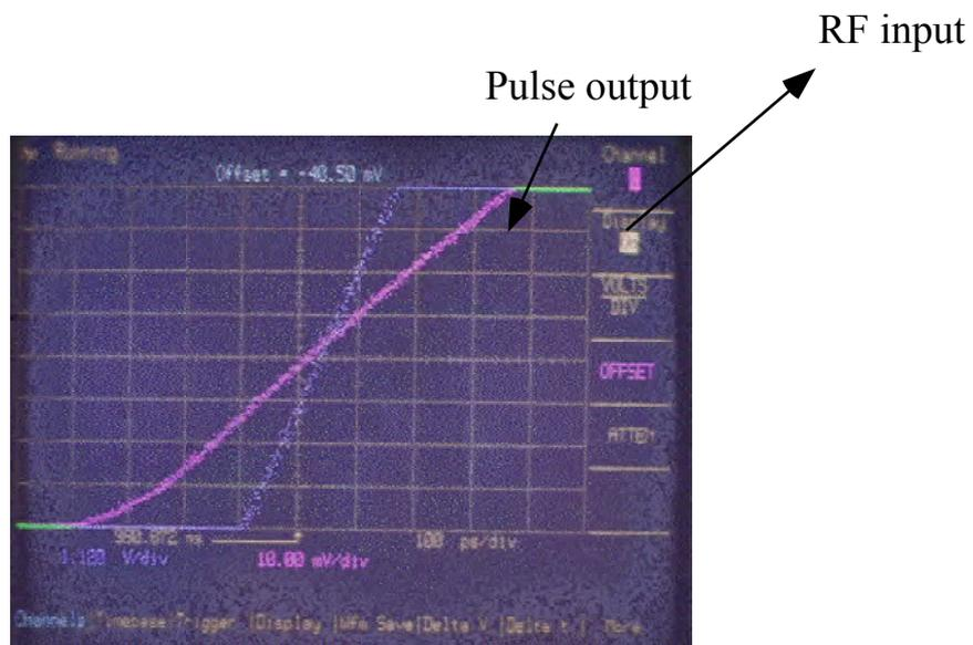
Showing the jitter with respect to 500MHz input (approx 10ps RMS)
