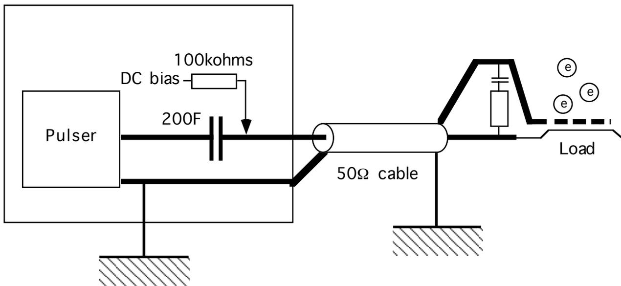
There is a resistor in series with a capacitor shown at the electron gun to make the load close to  $50\Omega$ . This must be chosen to minimise reflections up and down the connecting cable. (A typical value is  $100\Omega$ ).
