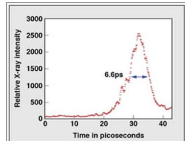
The time history of the X-ray emission from an experiment demonstrating sub-picosecond X-ray gating measured by the Dilation X-ray Imager.
