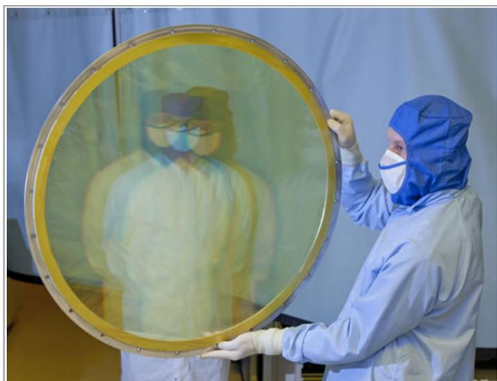
Mike Aasen holds the first diffractive membrane optic for the MOIRE imager. Multiple images of Tom Carlson appear behind the optic, which was designed and verified to achieve greater than 30 percent efficiency for the image used by the telescope.
